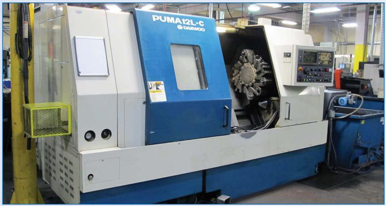
1996 **DAEWOO** PUMA12L-C CNC lathe with Fanuc OT CNC control, Travels: X-10.2", Z-41.3", 4.5" bar cap., 22.4" swing over bed (13.8" over carriage), 19" max. turning dia., 15" 3 jaw chuck (2,000 RPM), 12 station turret, tool presetter, programmable tail stock, intergrated steady rest, chip conveyor, sn PL120883
