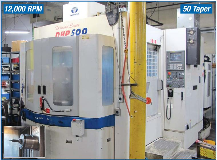
2000 **DAEWOO** DHP500 CNC horizontal machining centre, with FANUC 16M CNC control, Travels: X-33.4", Y-27.6", Z-29.5", (2) 19.7" x 19.7" pallets, 12,000 rpm, CAT 50, (60) ATC, 1,575 IPM, through spindle coolant, 0.1 deg. of indexing, 33HP, 1,760 lbs. pallet cap., chip blaster high pressure coolant, sn HP500027
