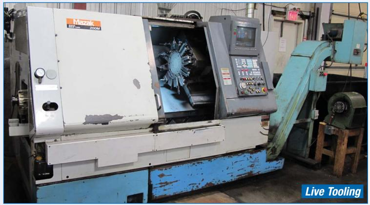
**MAZAK** SUPER QUICK TURN 200M CNC lathe with MAZATROL PLUS CNC control, Travels: X-6.55", Z-20.87", 2.06" bar cap., 11.8" max. turning dia., 8" chuck, 5,000 RPM, live tooling, tool presetter, chip conveyor, sn 136281
