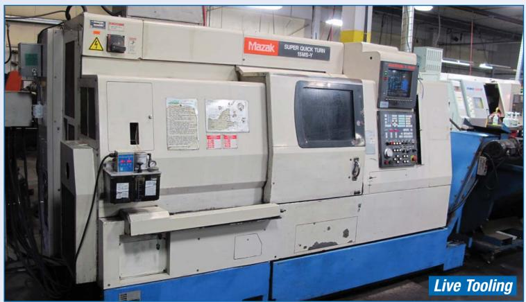
**MAZAK** SUPER QUICK TURN 15MSY CNC twin spindle lathe with MAZATROL PLUS CNC control Travels: X-7.1", Z-22.75", 2.4" bar cap., 20.9" swing over bed (11.81" over carriage), 8" chuck, 5,000 RPM, live tooling, tool presetter, chip conveyor, sn 112228. Note: sub spindle needs repair
